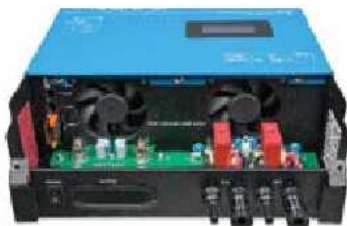
Inside the SmartSolar MPPT RS 450/100-AHC4
