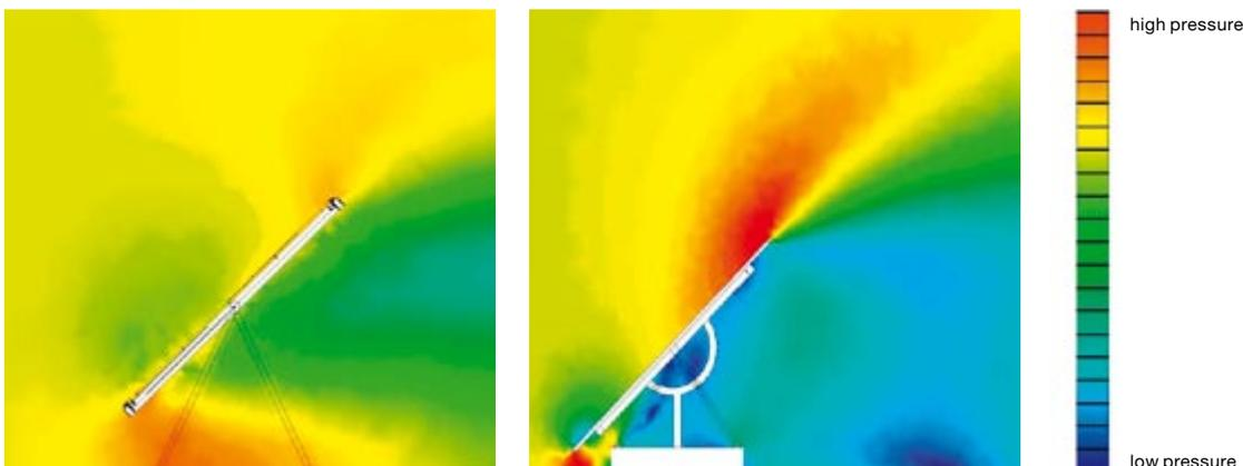
Comparison of wind flow simulations: SolarOptimus (left) and conventional tracking system (right). In case of conventional tracking systems large differences in pressure can be measured (heavy loads on system).
