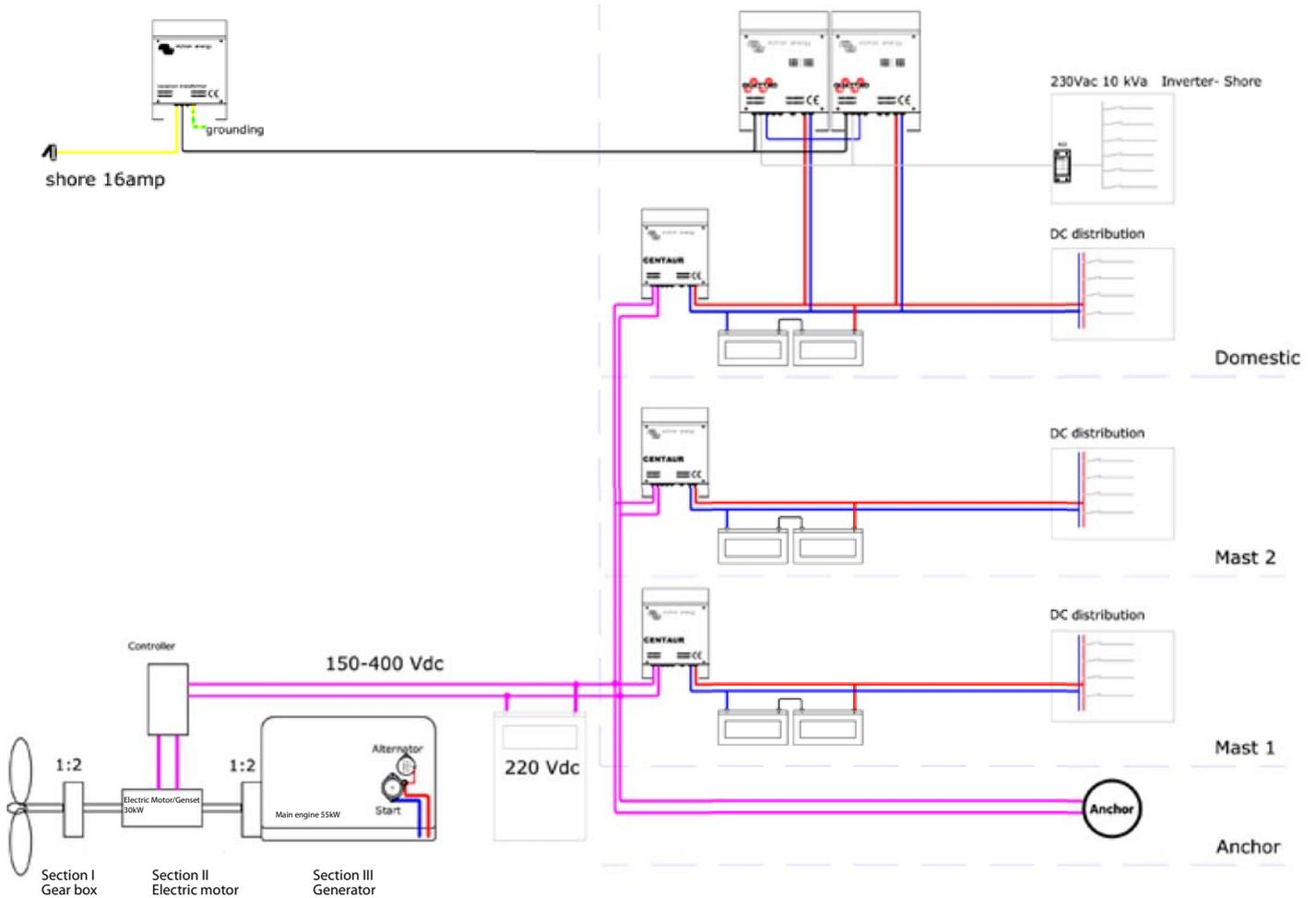
The drive system is highly redundant and consists of two identical "strings" of a mechanically coupled (bio) Yanmar diesel engine (55kW), a 20kW electrical motor/generator, a gearbox and a 'camber-adaptive' propeller. The sections I, II and III can be detached by couplings. Electrical power generation and electrical propulsion is provided by section I and II, while III and II provides a backup diesel generator function. Section I and III provides direct diesel propulsion.
