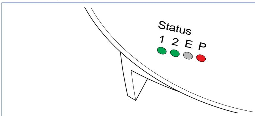
Depending on the operating status, LED 1, LED 2, and LED E can flash quickly or slowly, be permanently illuminated or not be illuminated.
