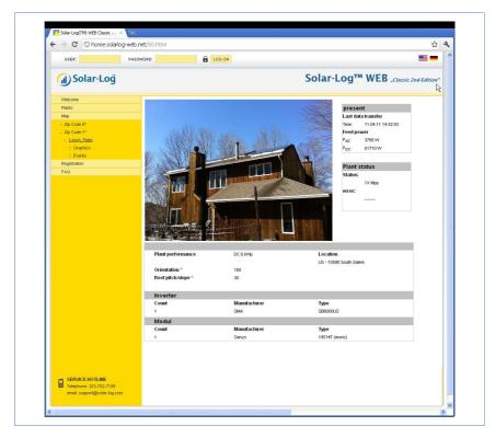
The detailed overview shows additional technical details about the plant as well as the plant status including any error messages that have occurred.
