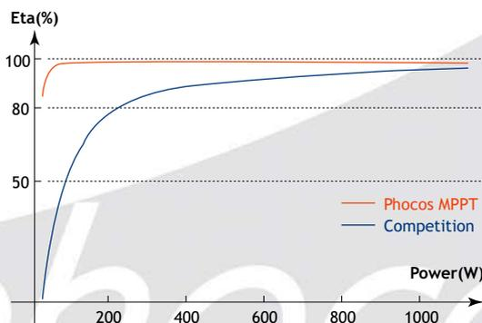
The Phocos MPPT100/30 was designed in order to yield all benefits of Maximum Power Point Tracking. Its efficiency is comparably high even on the lowest power levels. This means that the MPPT 100/30 keeps charging even in cloudy or rainy seasons where batteries cannot always be fully charged.
