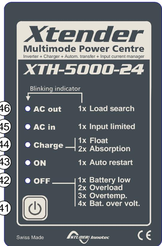
(42) This indicator lights up when the equipment has been stopped manually using the ON/OFF button (41). It also allows the cause of an unintentional stoppage of the device to be indicated via the different flashes, the imminence of a stoppage or the temporary limitation of its performance.
