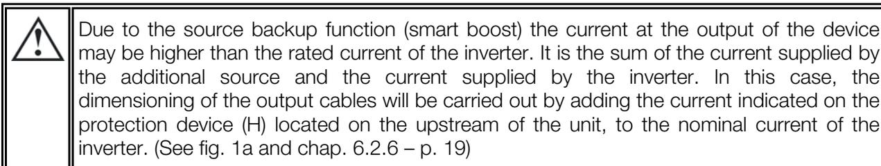
If the assistance function at the source (smart boost) is not used, the calibre of the protection device for the output (F) will be established at a maximum value equal to the rated current of the inverter, or at the maximum value of the protection device at the input (H) if this exceeds the rated current of the inverter.
