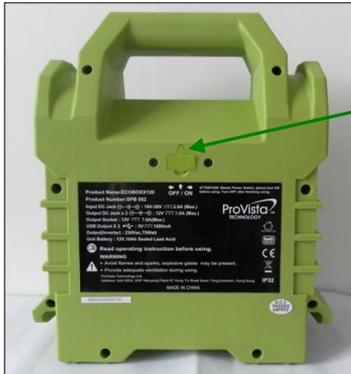
Lift up the rubber cap at the back of unit
