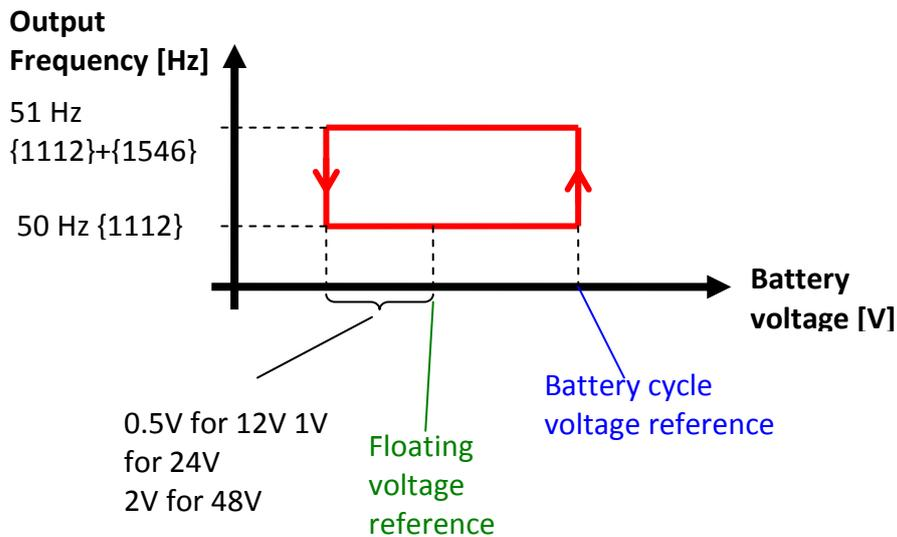
Figure 15: AC-output frequency behavior with a step when the battery is full for Xtender with param 1536
