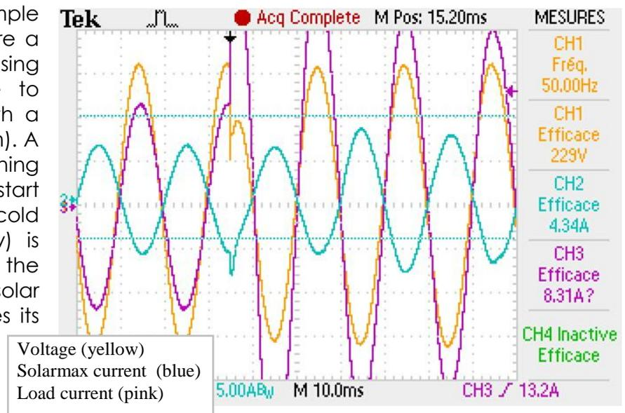
Figure 12: Big load transition on the system
