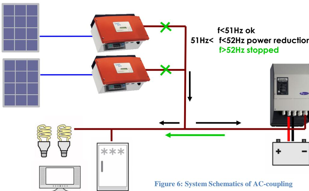
Figure 6: System Schematics of AC-coupling
