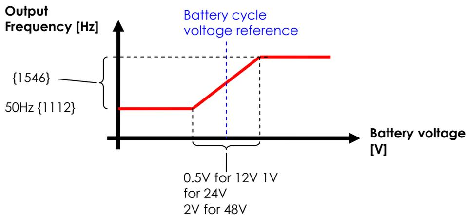
Figure 14: AC-output frequency behavior in function of the battery voltage for Xtender with param 1549
