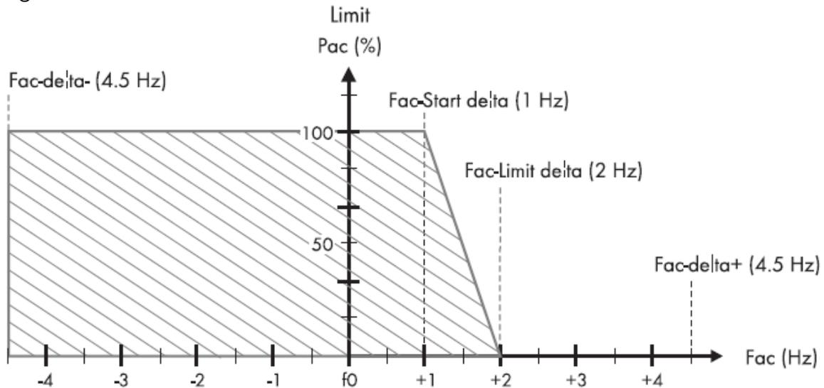
Figure 5: frequency shift power reduction as in SunnyBoy OFFGRID mode
