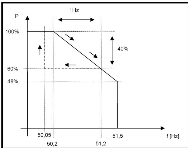
**Figure 3 : Frequency dependant power reduction as BDEW in KACO solar inverter**
