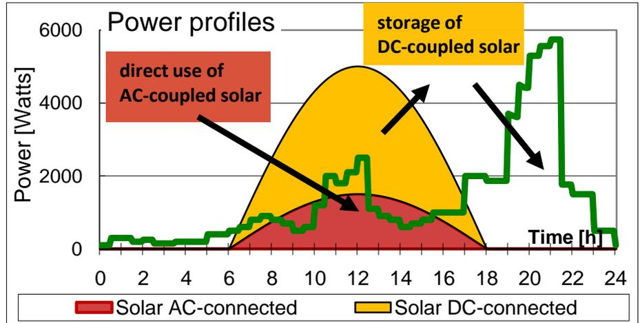
Figure 8: Split solar between AC and DC-coupling
