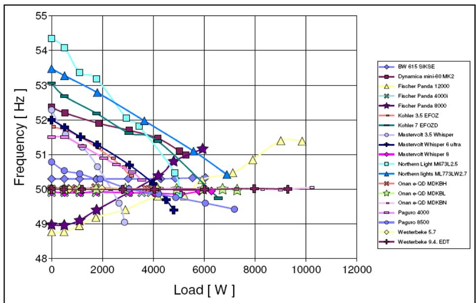
Figure 10: Frequency behavior of generators
