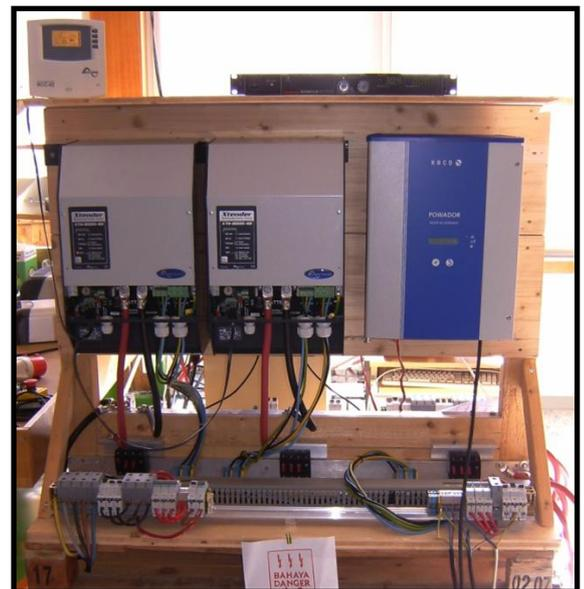
**Figure 4: Test bench with Kaco Powador**
