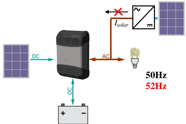
Figure 2 : AC-coupled solar inverter
