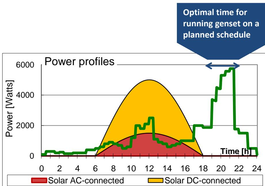
Figure 11: Best time to start a generator: when there is a load a no sun
