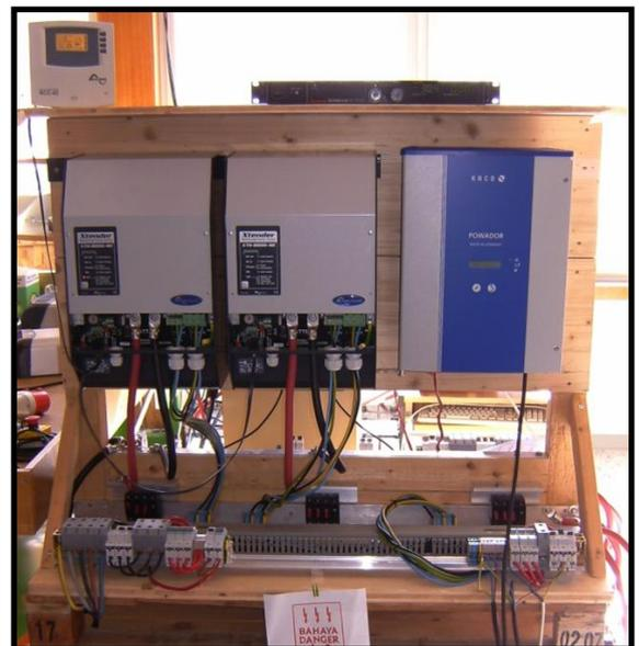
**Figure 4: Test bench with Kaco Powador**
