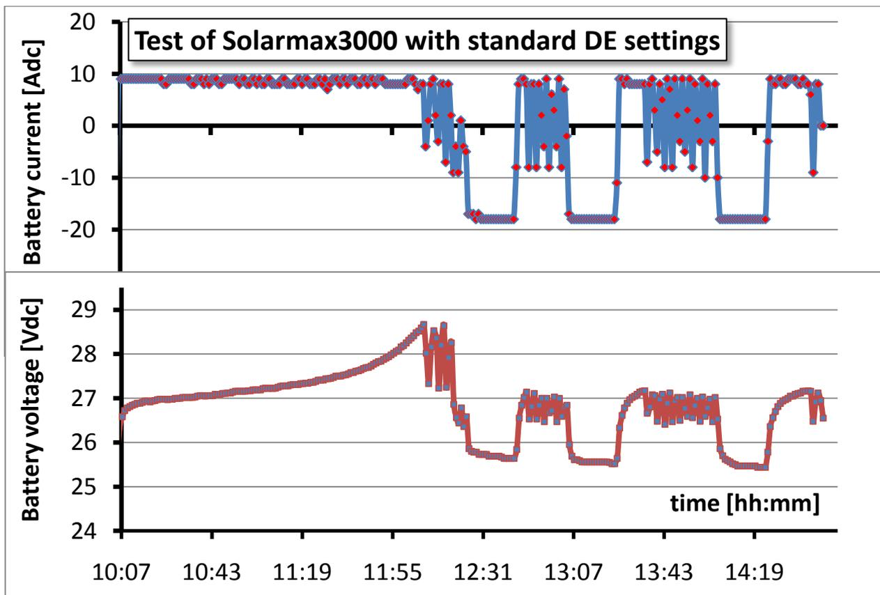
This behavior gives a less effective use of the AC-coupled solar during the top charge of the battery.
